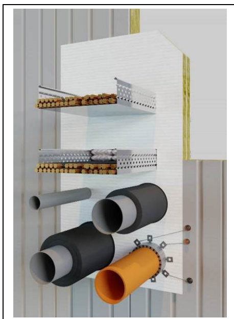
Figure A.3.4.1: Example of AF PANEL seal in a sandwich panels wall EI 120.
